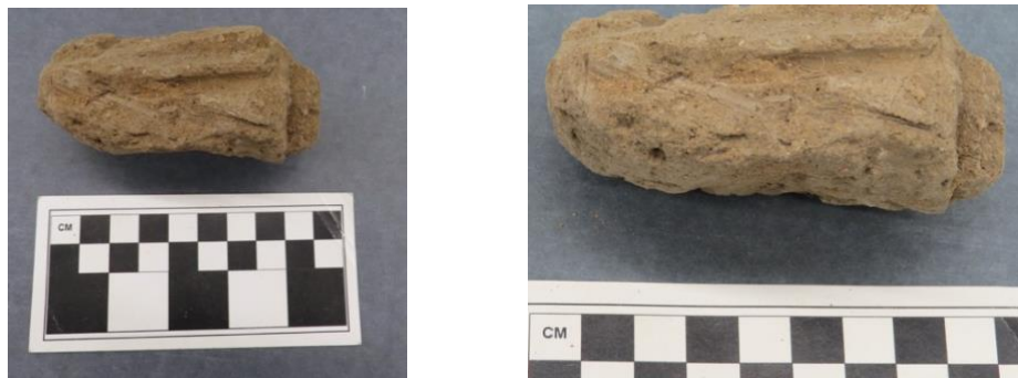
Figure 5.22. Adobe daub fragments. Left: Roofing daub with reed impressions. Right: Detail of reed impressions.
