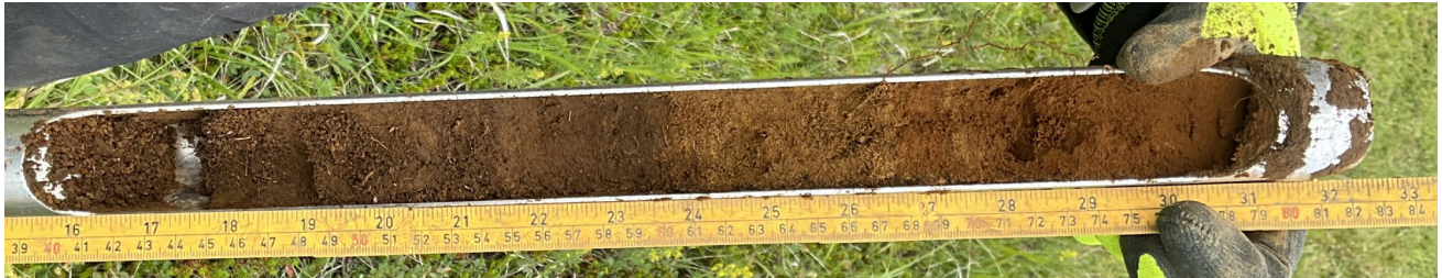
Figure 12. Core 241243, showing the transition at approximately 60cm bgs between two types of turf.
