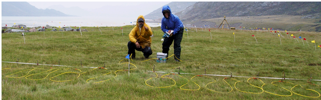
Figure 7. Electrical resistivity surveying with Syscal Kid meter.
