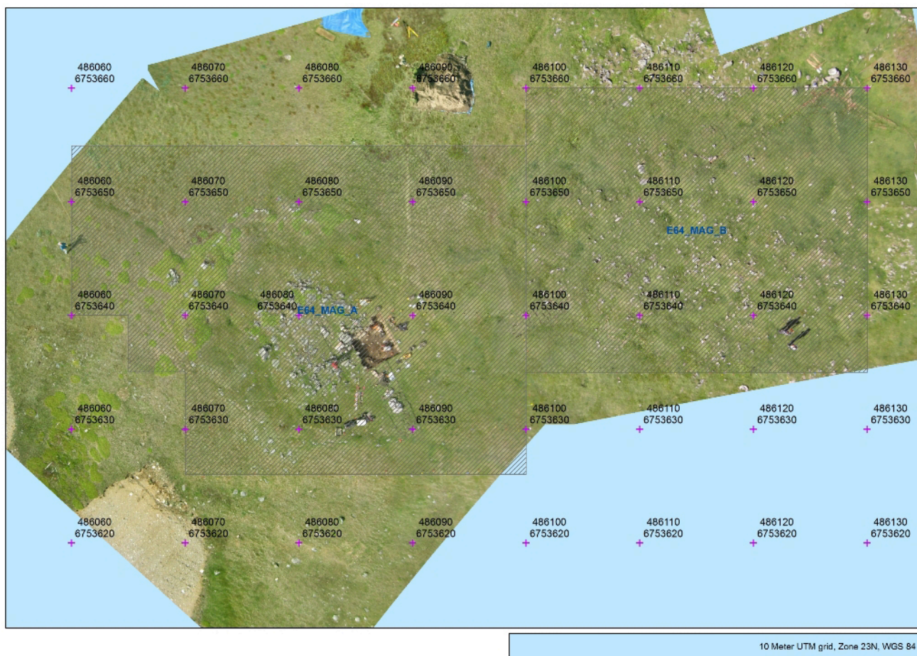
Figure 28. Ø64 Location of magnetic surveys (hatched areas). Magnetometer surveys were conducted in two conjoined areas, one centered over the churchyard, the other centered over the medieval farm ruins.
