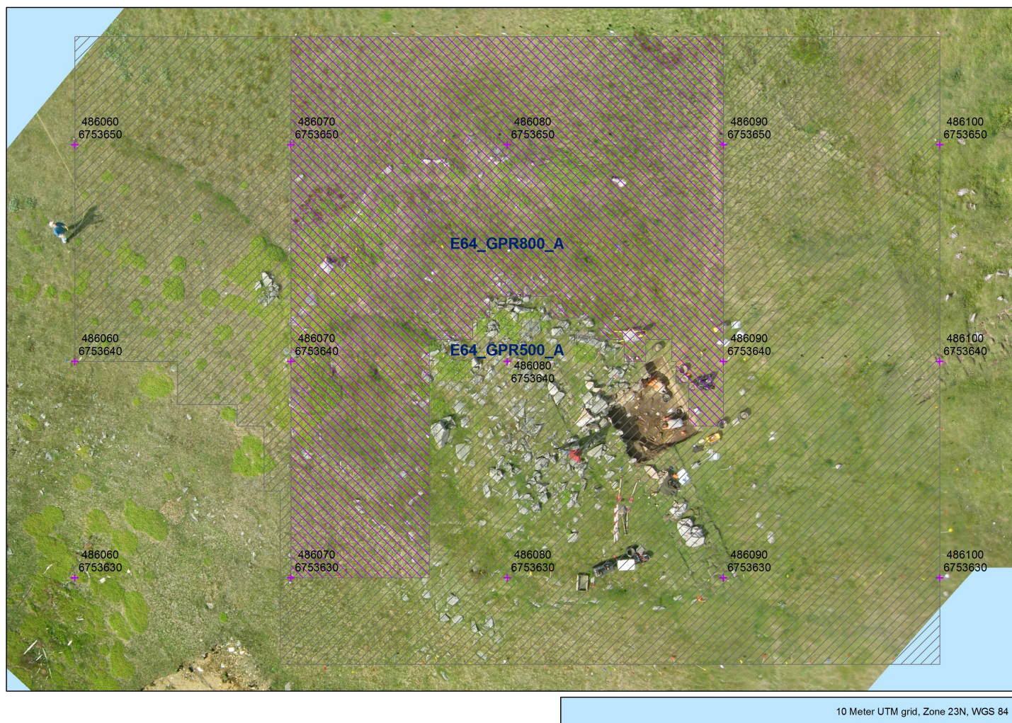
Figure 19. Ø64 Location of GPR survey (hatched area). GPR radargrams and time slices are incorporated into the text
