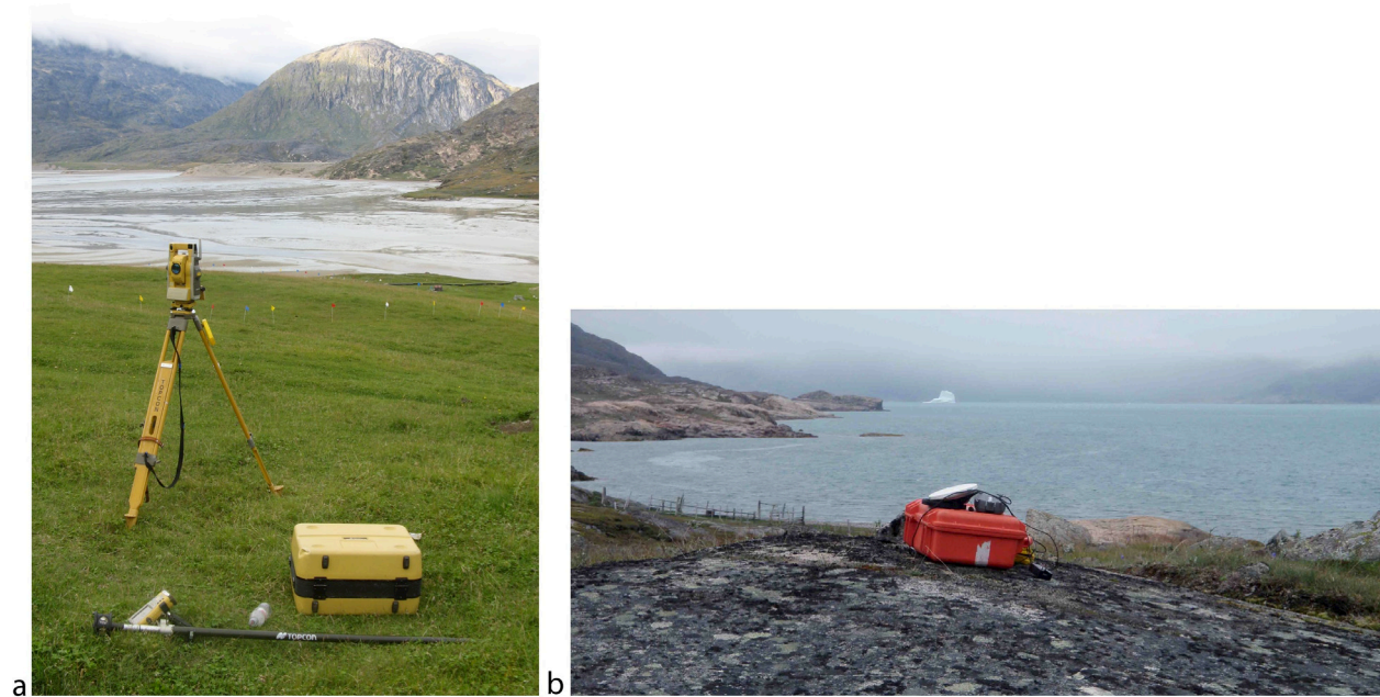
Figure 1. Survey grid establishment: (a) GPT9005A robotic total station, and (b) Trimble GeoXH GPS with a Zephyr antenna.
