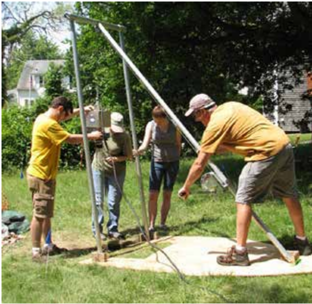
Figure 7. Setting up the VibeCore on the Jenney Pond lot. This was used to core in the bottom of deep shovel test pits.
