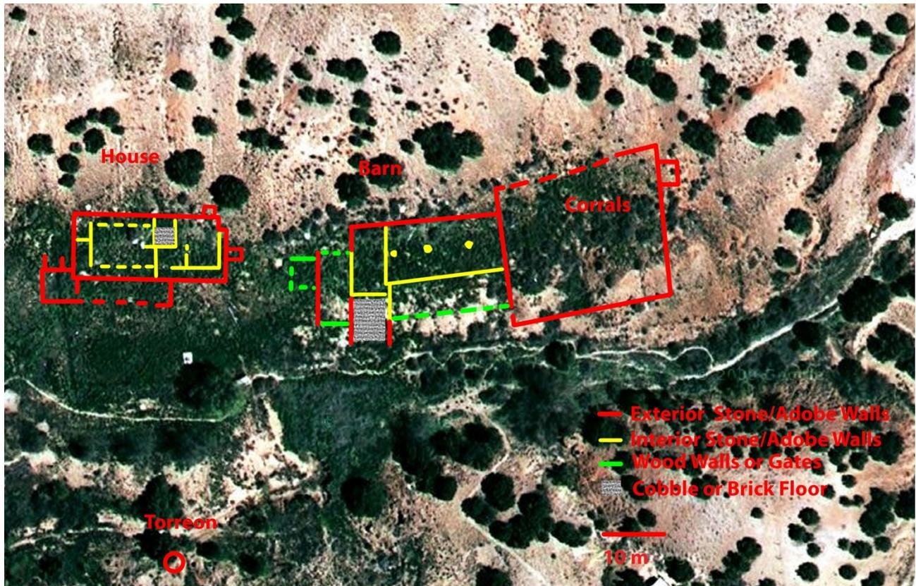
Figure 76. Hypothetical reconstruction of the floor plan at LA 20,000. Dashed lines are hypothesized walls, rather than verified walls. Red lines are exterior stone and adobe walls; yellow lines are interior stone and adobe walls; green lines are wooden walls or gates.
