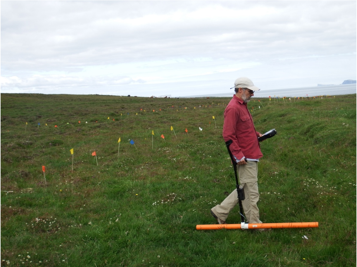
Figure 4. Using the CMD Mini Explorer with the boom oriented parallel to the direction of transects.
