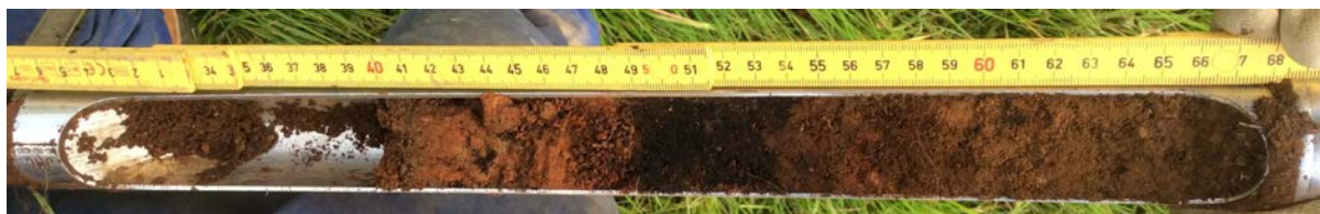
Figure 16. Second barrel of core 174349 showing distinct turf deposit form 49-54 cm bgs
