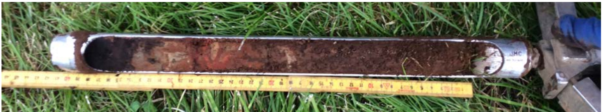
Figure 11. Core 171492 showing floor from 33 cm bgs with turf above it.
