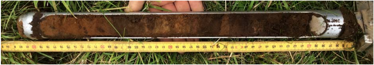
Figure 9. Second barrel of core 171488 showing distinct turf deposit form 35-67 cm bgs
