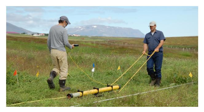
Figure 7. Electromagnetic surveying with the DualEM-21 (pictured at Stóra-Seyla). Damiata, keeps track of the distance, while Steinberg right, pulls unit at an even pace along the ground surface.
