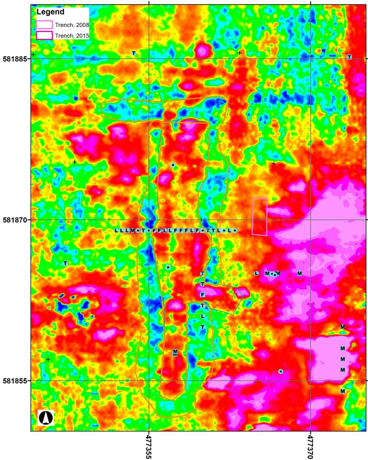
Figure 28. 2016 CMD Explorer IP3 with pre-1104 coring results test trenches, and potential outline of structure.
