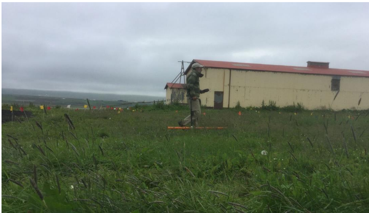
Figure 13. Using the CMD Mini-Explorer at Egg.
