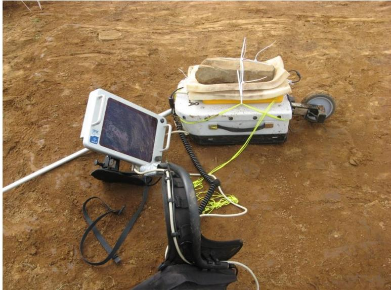
Figure 12. Photograph of the Mala X3 equipped with a 500 MHz antenna.
