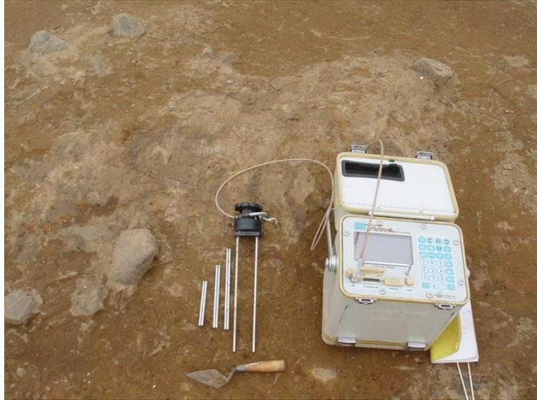
Figure 11. Photograph of the Trase 6050X1 TDR instrumentation.
