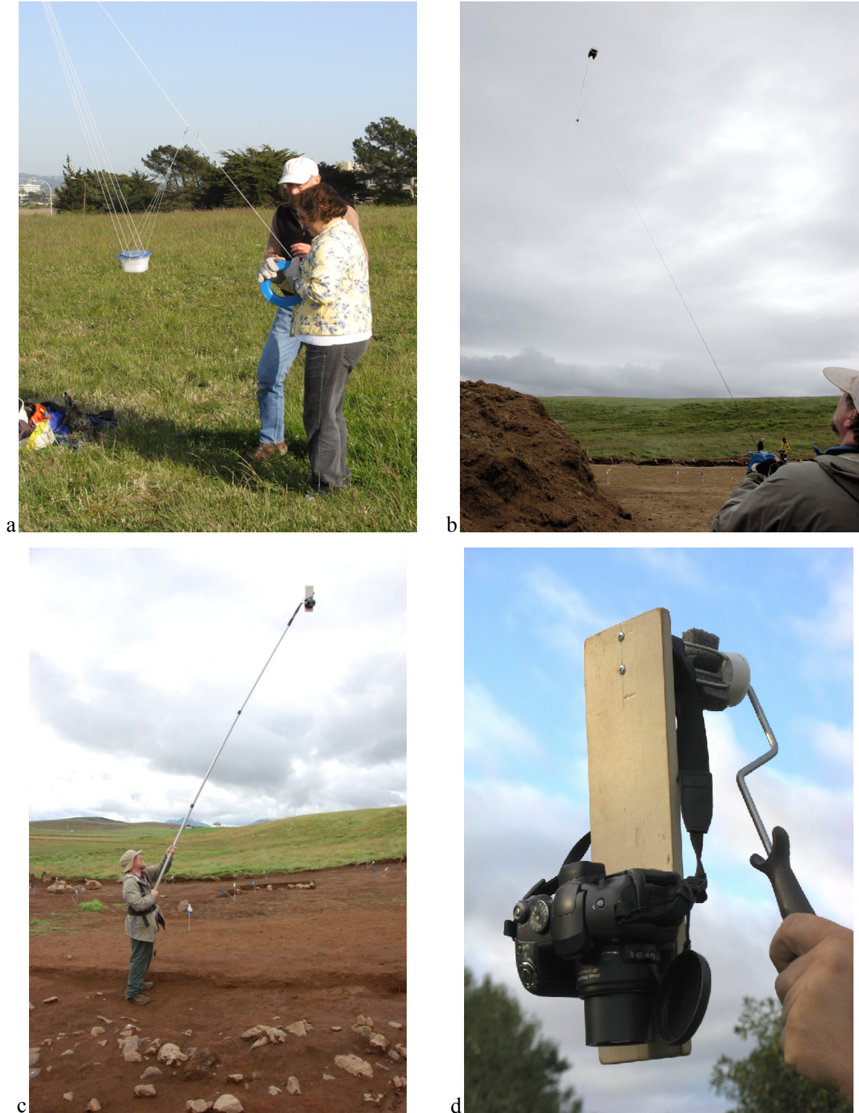
Figure 5. (a) KAP camera box, (b) kite in flight Stóra-Seyla, (c) pole-based photography, and (d) detail of pole-based camera mount.
