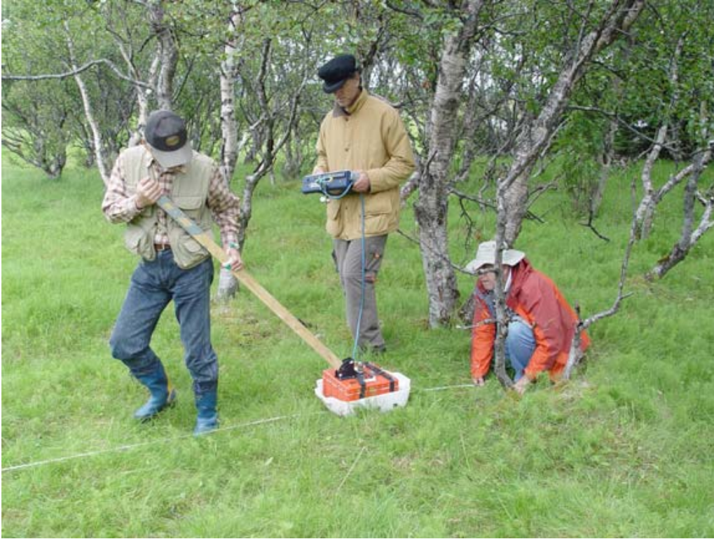
Figure 15: Using the 400 MHz antenna.
