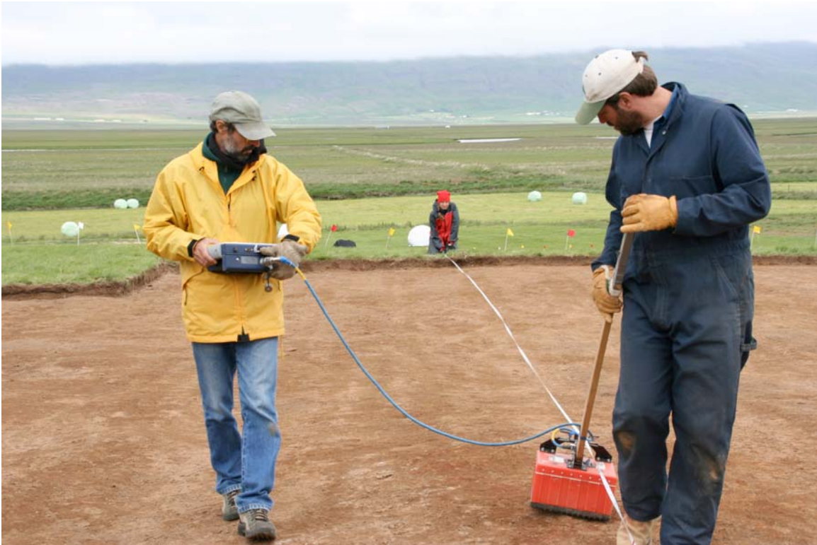
Figure 25: Using the 400 MHz antenna at Glaumbaer.
