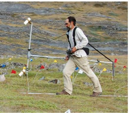
**Conductivity:** sends an alternating current into the ground and measures the resulting magnetic field. Results have two components, the bulk conductivity and the in-phase.
