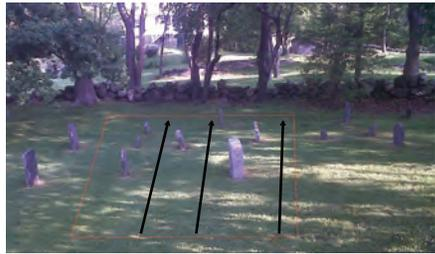
**Transect:** Most geophysical instruments record lines of data. Along these transect lines, data is recorded with specific coordinates.
